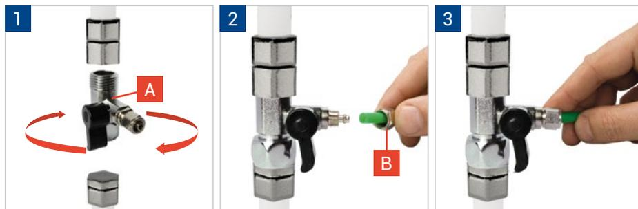
2. Insert a plastic pipe (Fig. 2) into a screw (B). Insert a pipe into a fitting of a ball valve until it stops and tighten a screw (рис. 3).
